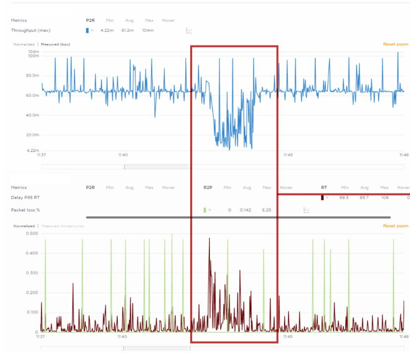
Normally, during business days, the network can display burstiness (as shown with the throughput in blue). But in the specified window of time, Farmers & Merchants experienced network downtime. This was because the end result of packet loss and delay is reduced network throughput, resulting in poor performance.
