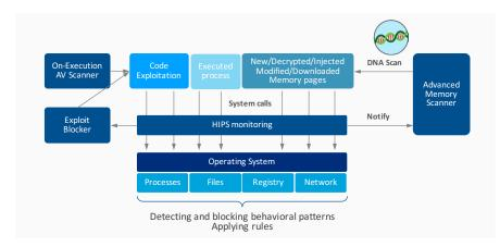
Fig.2: How ESET's behavioral detection works
